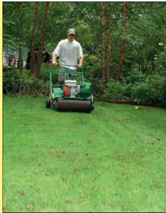
Core aerator pulls plugs from the entire lawn.
