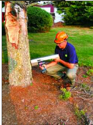
A Resistograph measures and records the variations in wood strength and allows the detection of decay within trees.
